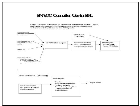
The above figure, "SNACC Compiler Use in SFL", demonstrates the eSNACC compiler use. First, the .cpp and .h source files are built from an ASN.1 specificaion (file) using the eSNACC compiler, then the main application is built using these support files and the eSNACC run-time library. The application program can encode/decode ASN.1 data and reference individual elements using the eSNACC run-time library classes described in this manual.
